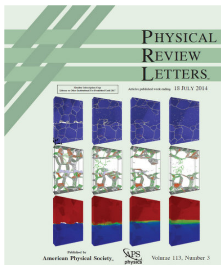
Figure 2.18: Snapshots of the evolution of sliding contact between two nanocrystalline iron tribopartners. Each column presents the instantaneous state of the grain structure (top panel), the grain boundaries and dislocations (middle panel), and the corresponding sliding interface (bottom panel) at selected sliding times.
