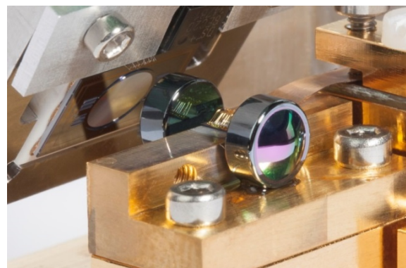
Figure 2.22: Rapid-scanning quantum cascade laser in external cavity configuration employing a resonantly driven MEMS grating for wavelength-selective optical feedback.
