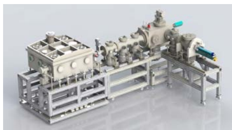
Figure 1.14: Storage ring setup for photoelectron spectroscopy on size-selected clusters currently commissioned at the TICNN, Tianjin, China.
