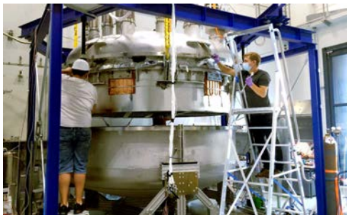
Figure 3.19: The new LXe detector test platform in the astroparticle physics laboratory in Freiburg.
