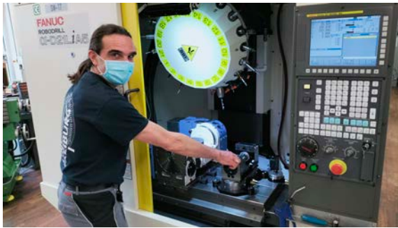
Figure 1.5: 5-axis milling center in the Mechanical Workshop at the Institute of Physics.
