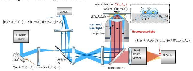
Schematic of a ROCS imaging system: Partially coherent images from back-scattered laser light are combined by rotation in the azimuthal angle  $\varphi$  change with the incident k-vector, which can be controlled by the the laser wavelength  $\lambda$  and the polar angle  $\beta$  of incidence. Fluorophores delay the phase of the backscattered laser light and emit fluorescence light at the same time for object identification and control.
