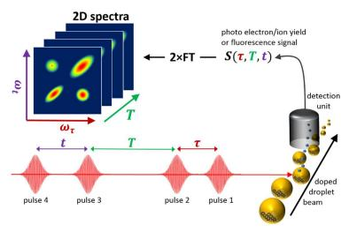
and energy transport in simple, isolated donor-acceptor-systems. With multidimensional coherent spectroscopy the sample is illuminated by a sequence of several precisely controlled ultra-short laser pulses, and the induced processes are detected by means of fluorescence, photoelectron or photoion yields. In particular, this allows us to directly observe coherent dynamics.
